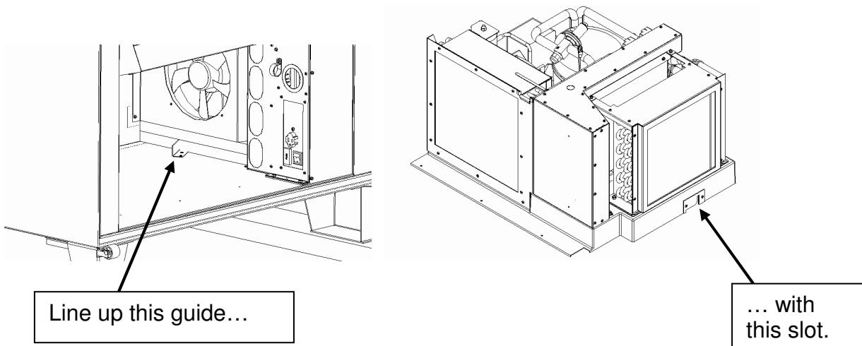
2. Insert the wedge tabs into the slots in the refrigeration base plate the cabinet.
