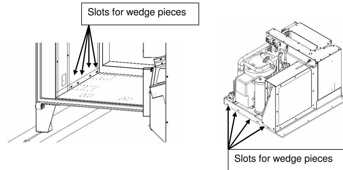
1. Use a rubber hammer and flatten the wedges. Bend should go past center.
