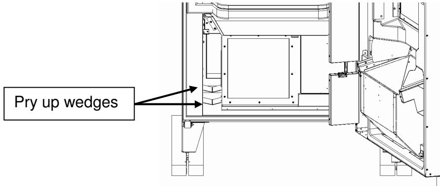
5. Slide the refrigeration unit to the left and then pull out. Do not try to loosen the unit if it is frozen to the cabinet. Allow to thaw thoroughly first.
